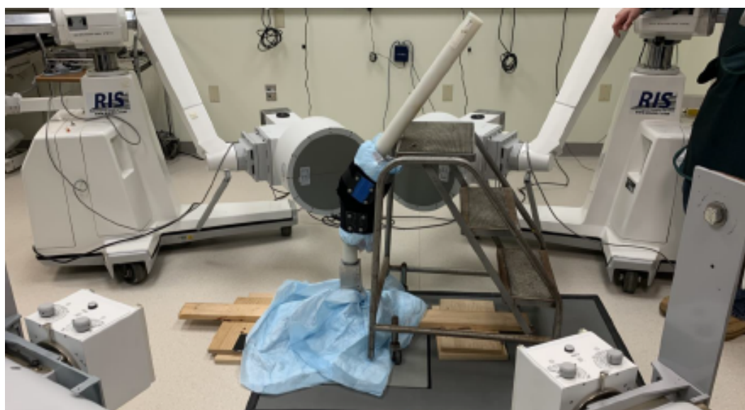
Figure 2: Image from the morning of the experiment showing the cadaver leg, outfitted with reflective skin markers, inside the DF-MBT system.
