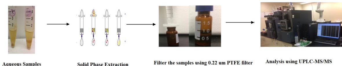
**Figure 3.5**-TrOCs extraction from aqueous fraction of BS slurry
