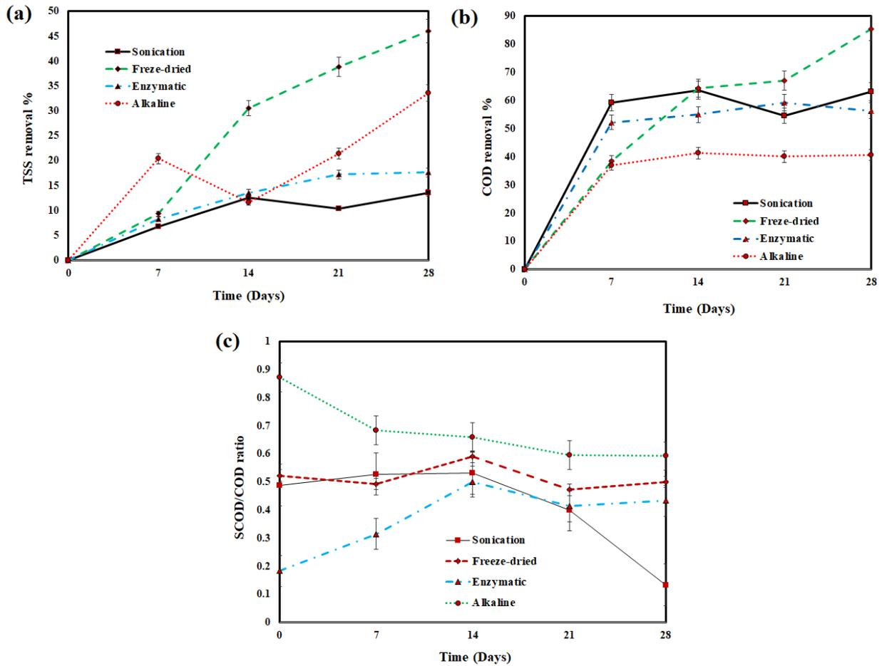
**Figure 5.4-** (a) TSS removal (b) COD removal and (c) SCOD/COD ratio of after bioaugmentation of *B. subtilis* with pre-treated biosolids after 28 days
