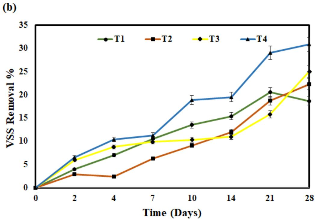
**Figure 4.4-** Removal of a) TSS and b) VSS during the digestion of biosolids slurry by various treatments (T1 – T4).
