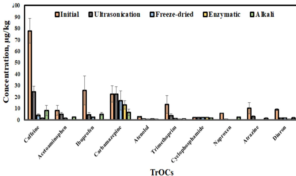
**Figure 9-** TrOCs concentration after bioaugmentation of *B. subtilis* with pre-treated biosolids after 28 days in solid phase. (Initial: Caffeine-77.2±10.8 µg/kg, Acetaminophen-8.2±4.2 µg/kg, Ibuprofen-25.6±12.7 µg/kg, Carbamazepine-22.6±7.0 µg/kg, Atenolol-2.6±0.5 µg/kg, Diuron-8.8±0.8 µg/kg, Atrazine-10±4.9 µg/kg, Naproxen-5.6±0.5 µg/kg, Cyclophosphamide-2.0±0.0 µg/kg, Trimethoprim-13.4±7.6 µg/kg).
