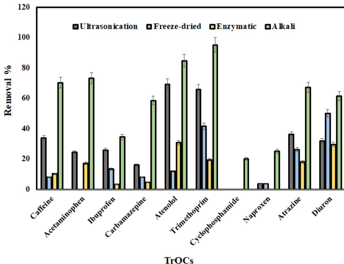
**Figure 5.3-** TrOCs removal after pretreatments in solid fraction of biosolids slurry
