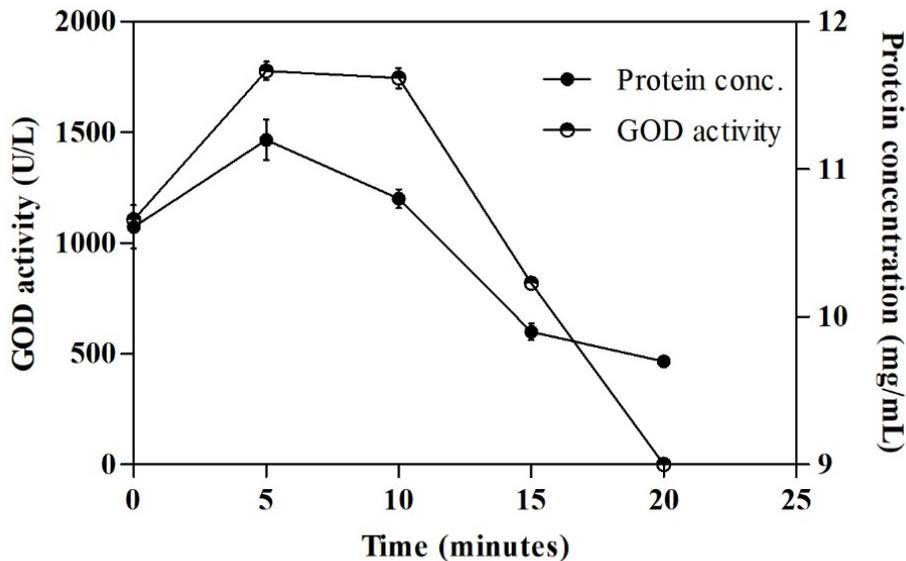
**Figure 6.5-** Effect of ultrasonication on recovery of GOD. Protein concentration (mg/mL) and GOD activity (U/L) during ultrasonication of 25% (dw/v) BS slurry for GOD production, with respect to time during sonication for 25 minutes. All studies were conducted in triplicates and reported as average along with the standard deviation.
