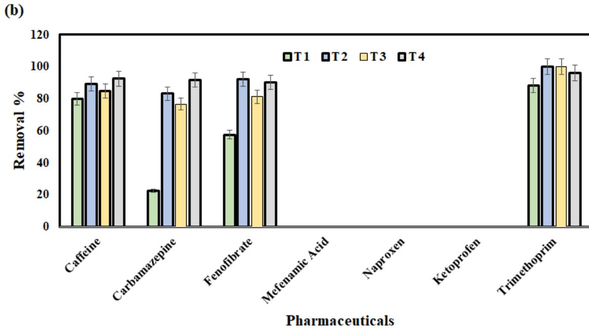
**Figure 4.2-** Removal of pharmaceuticals in (a) solid, and (b) aqueous phase during digestion of biosolids slurry by various treatments (T1 – T4).
