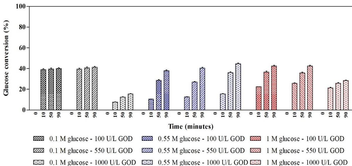
**Figure 11-** Glucose oxidation using BS-based GOD. (a) Glucose conversion obtained with different concentrations of glucose with varying activities of GOD; (b) Hydrogen peroxide concentration obtained with different concentrations of glucose with varying activities of GOD.
