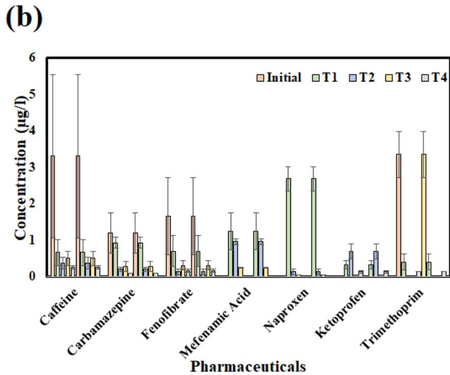
**Figure 5-** Concentration of pharmaceuticals in (a) solid, and (b) aqueous phase during digestion of biosolids slurry by various treatments (T1 – T4)
