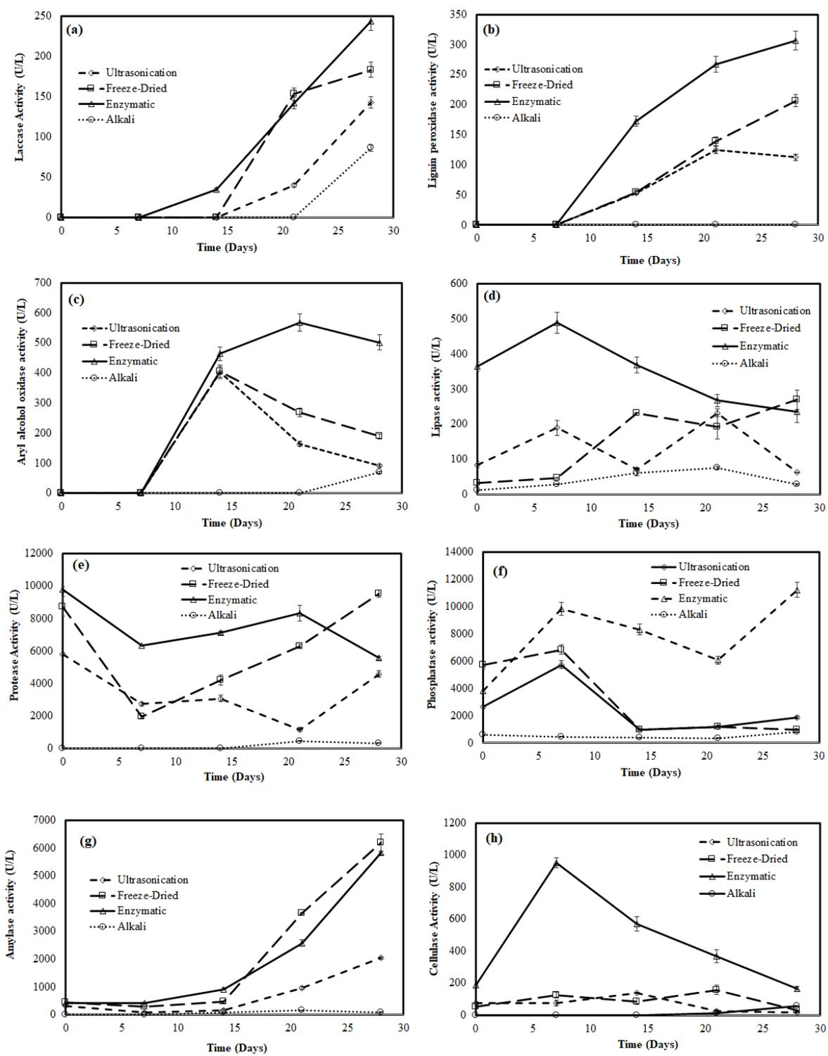
**Figure 5.5-** Extracellular enzyme profile during bioaugmentation of *B. subtilis* with pre-treated biosolids. ((a) laccase, (b) lignin peroxidase, (c) aryl alcohol oxidase, (d) lipase (e) protease (f) phosphatase (g) amylase and (h) cellulase).
