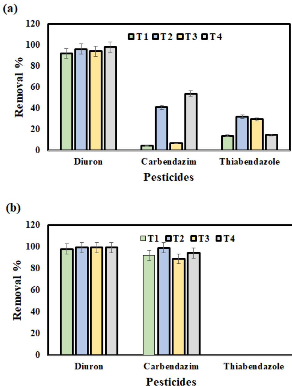
**Figure 4.3-** Removal of pesticides in (a) solid and (b) aqueous phase during digestion of biosolids slurry by various treatments (T1 – T4).
