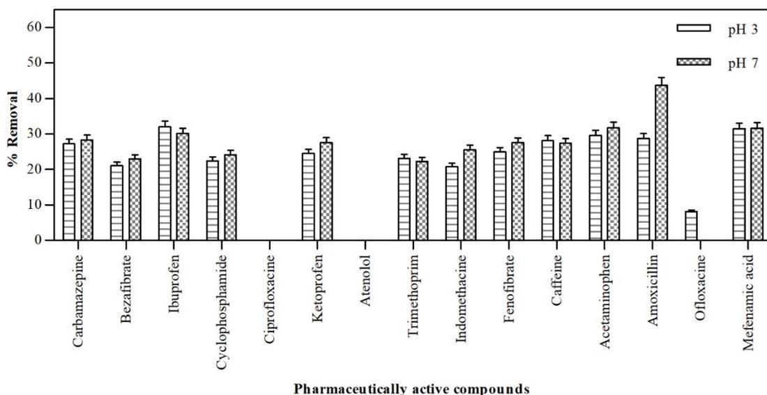
**Figure 6.6-** Effect of pH on removal of PhACs from aqueous solutions using bio-Fenton oxidation. The removal of the 15 PhACs existing as mixtures in aqueous solutions at a concentration of 500  $\mu\text{g/L}$  (each) and  $[\text{H}_2\text{O}_2:\text{FeSO}_4]$  of 50:1 at acidic (pH 3.0) and neutral pH (pH 7.0). All studies were conducted in triplicates and reported as average along with the standard deviation.
