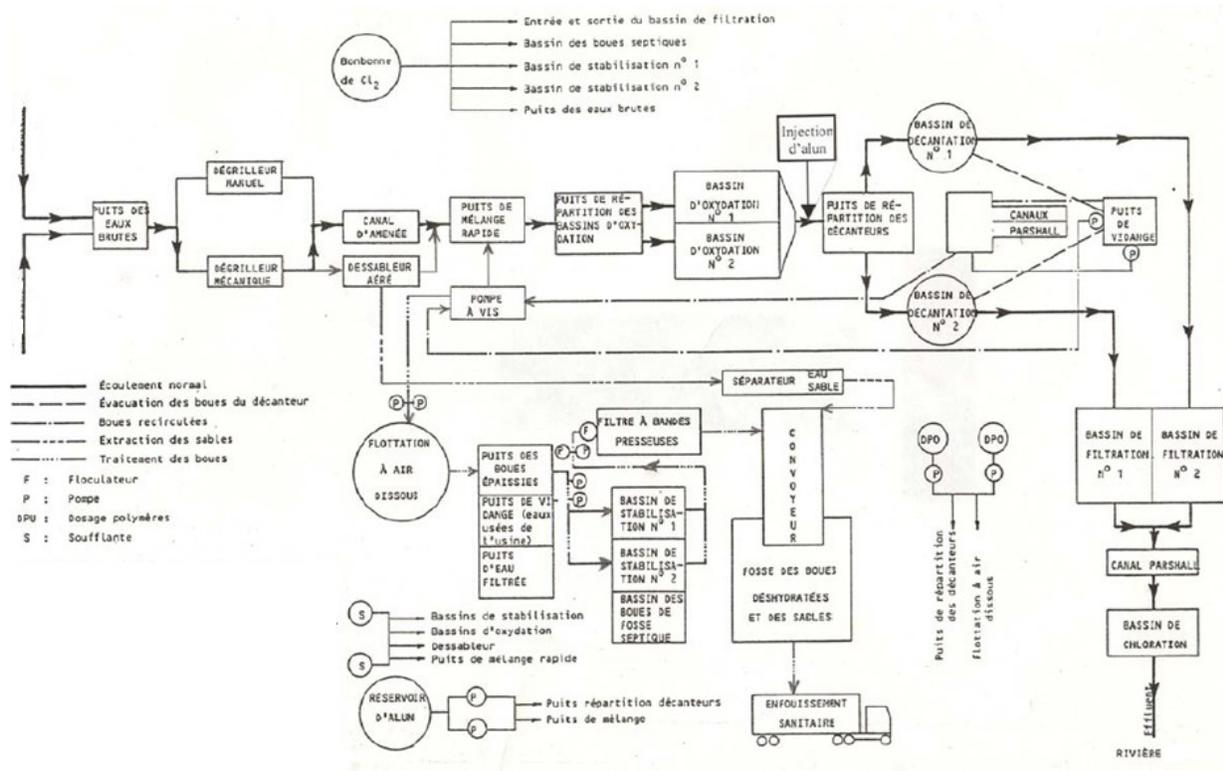
Figure 3.1- Wastewater and sludge treatment line of municipal WWTP
