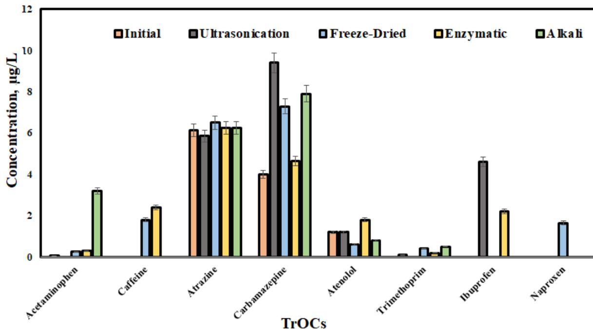
**Figure 10-** TrOCs concentration after bioaugmentation of *B. subtilis* with pre-treated biosolids after 28 days in aqueous phase. (Initial: Caffeine-ND, Acetaminophen- $0.05 \pm 0.05$   $\mu\text{g/L}$ , Ibuprofen-ND, Carbamazepine- $4 \pm 2$   $\mu\text{g/L}$ , Atenolol- $1.2 \pm 1.2$   $\mu\text{g/L}$ , Atrazine- $6.1 \pm 0.2$   $\mu\text{g/L}$ , Naproxen-ND, Trimethoprim- $0.1 \pm 0.1$   $\mu\text{g/L}$ ).
