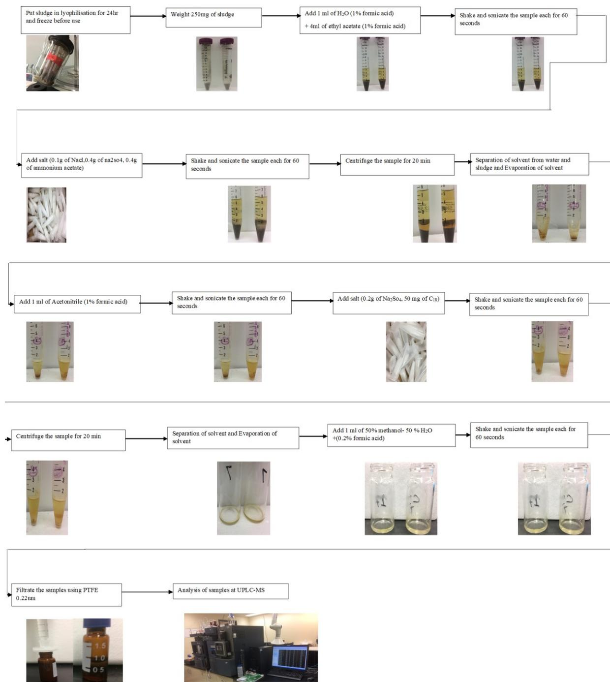
**Figure 3.4-TrOCs extraction from solid fraction of BS slurry**
