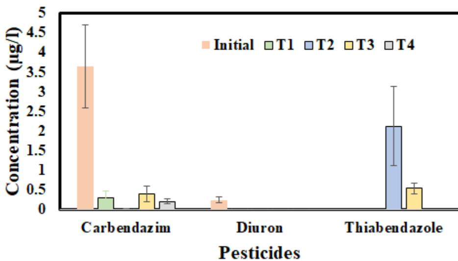
**Figure 6-** Concentration of pesticides in (a) solid and (b) aqueous phase during digestion of biosolids slurry by various treatments (T1 – T4)
