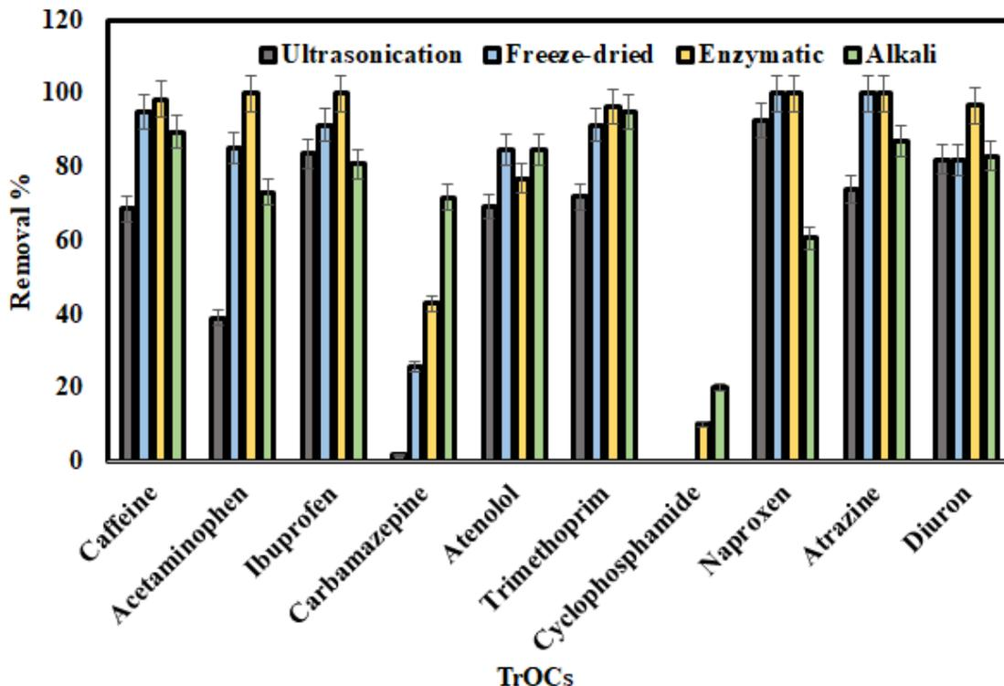
**Figure 5.6-** TrOCs removal after bioaugmentation of *B. subtilis* with pre-treated biosolids
