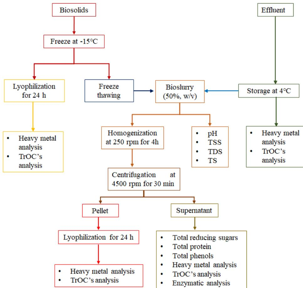
Figure 3.2- Schematic diagram of preparation and characterization of BS slurry
