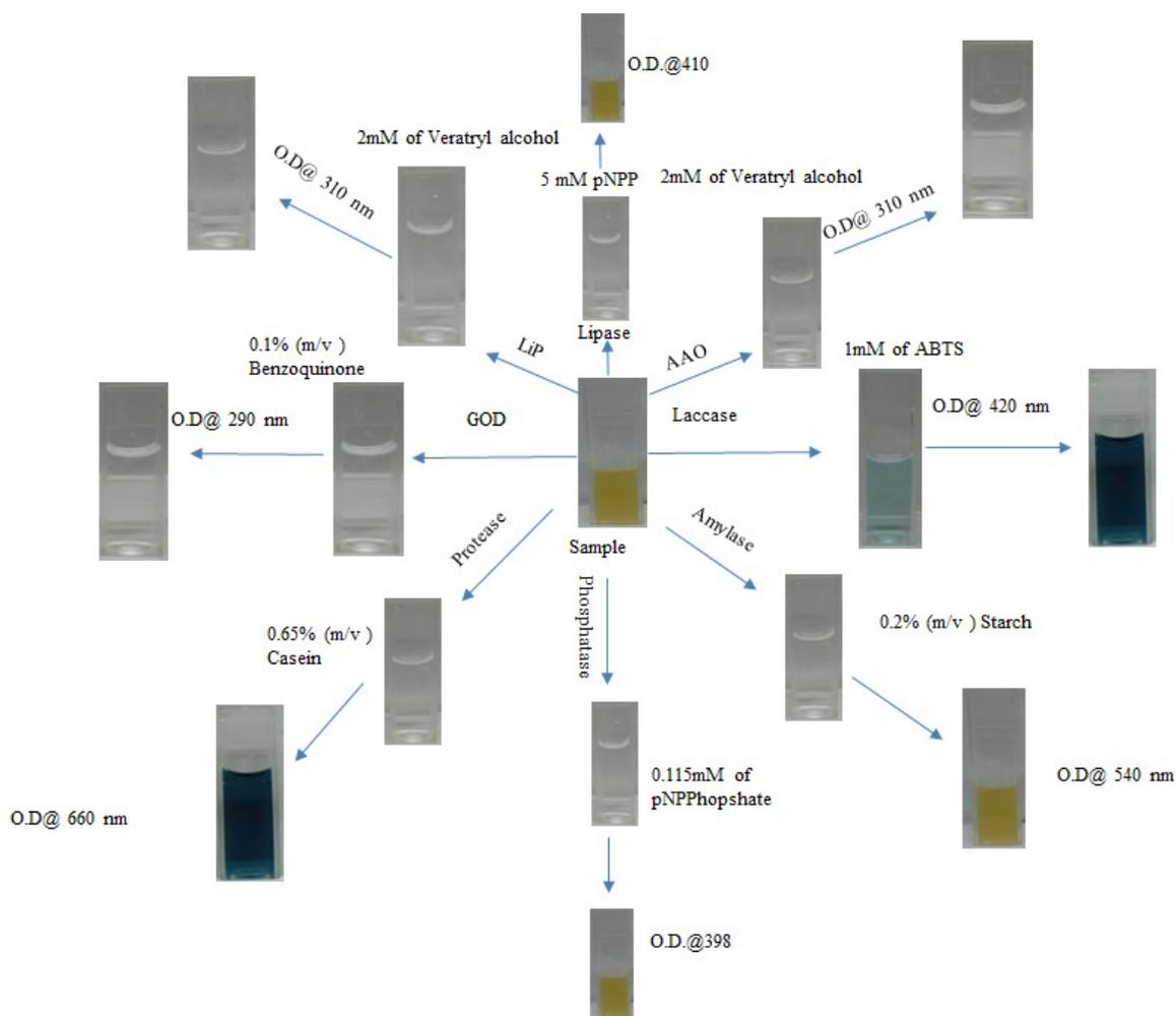
Figure 3.3- Various enzyme assays measured in BS slurry
