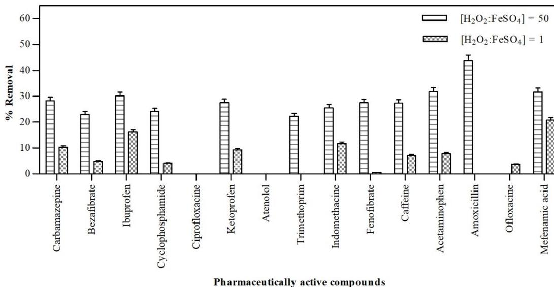
**Figure 6.7-** Effect of  $[\text{H}_2\text{O}_2:\text{FeSO}_4]$  on removal of PhACs from aqueous solutions using bio-Fenton oxidation. The removal of the 15 PhACs existing as mixtures in aqueous solutions at a concentration of  $500 \mu\text{g/L}$  (each) and neutral pH (7.0) at varying  $[\text{H}_2\text{O}_2:\text{FeSO}_4]$  of 50:1 and 1:1. All studies were conducted in triplicates and reported as average along with the standard deviation.
