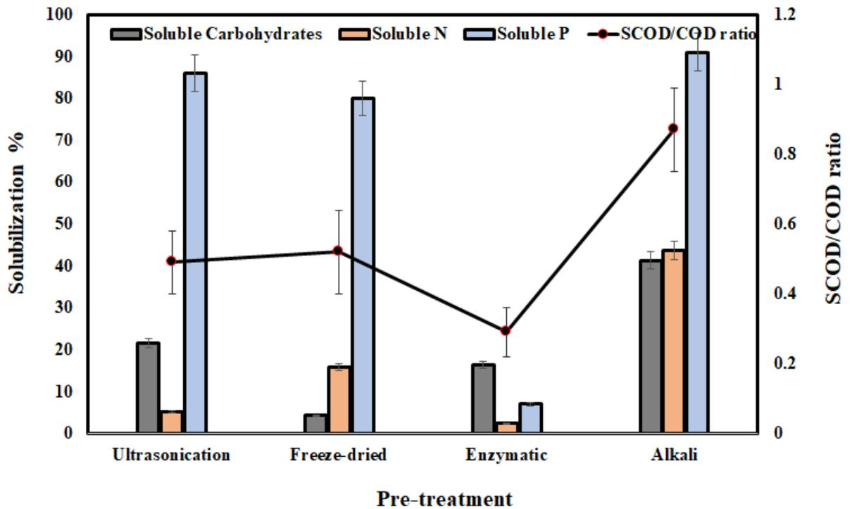
**Figure 5.1-** Impact of various pretreatment methodologies on nutrient parameter of biosolids. (Initial SCOD/COD ratio of  $0.26 \pm 0.03$ , soluble N, P and Carbohydrate concentrations are  $34.09 \pm 0.7$  mg N/L,  $14.1 \pm 3.9$  mg P/L and  $94.9 \pm 15$  g/L, respectively).
