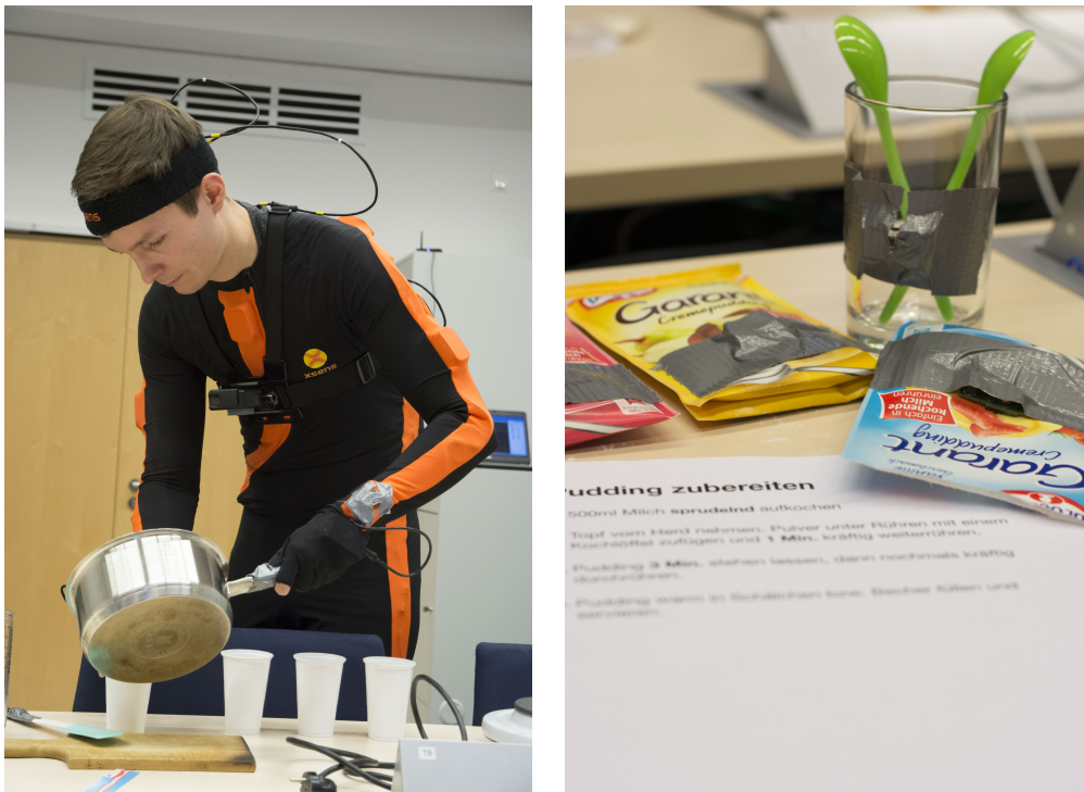
Figure 1: During recording of the Kitchen Task setting. Test subject is equipped with Motion Capturing Suit, ECG, EDA, and chest mounted camera (left). Objects were instrumented with custom BLE wireless motion sensor platform (right).
