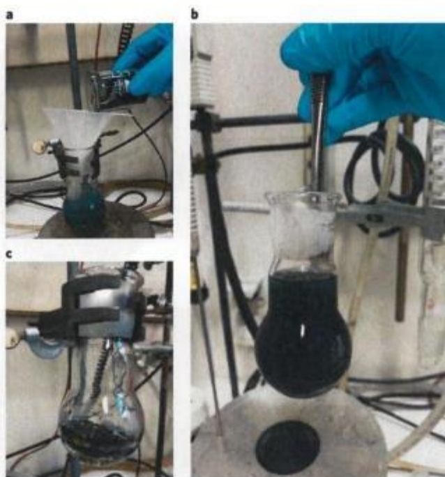
Fig. 15 | Impregnation of Co-DABCO-TPA MOF on carbon. a-c. Addition of Vulcan XC72R carbon black support (a); after addition of Vulcan XC72R carbon powder support (b); after 20 h of drying by slow solvothermal process (c).
