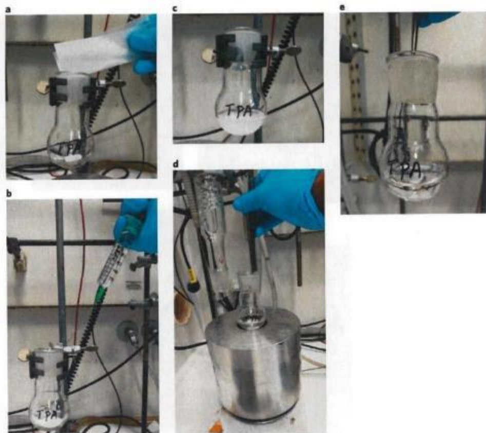
Fig. 13 | Preparation of TPA solution in DMF. a–e , Addition of TPA to the other RB flask ( a ); addition of DMF to TPA in RB flask ( b ); after addition of DMF to TPA at room temperature ( c ); placing the undissolved TPA in the aluminum block for heating at 150 °C for 5 min with stirring ( d ); TPA solution after 5 min of heating at 150 °C ( e ).
