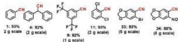
Scheme 6 Demonstrating the gram scale reactions for the synthesis of some selected nitriles over the \text{Fe}_2\text{O}_3 -N/C catalyst. Reaction conditions: 2–5 g substrate, the weight of the catalyst corresponds to 3 mol% Fe, 200 \mu\text{L} aq. \text{NH}_3 for every 0.5 mmol substrate, 40 ^\circ\text{C} , 10–50 mL t -amyl alcohol, 1 bar \text{O}_2 (balloon), 24–30 h. Isolated yields are shown.
