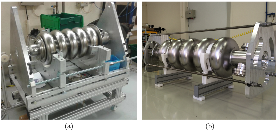
Fig. 3.1. Bulk Nb prototypes of (a) the medium- \beta SPL cavity [23] and (b) the high- \beta SPL cavity.
