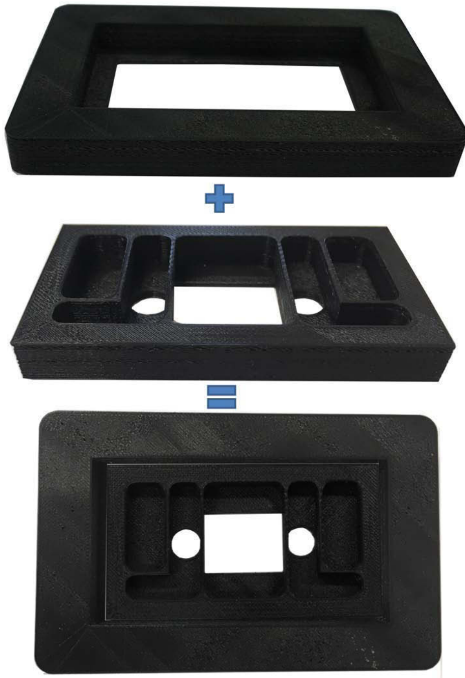
Figure 4.2: 3D printed electro-taxis chamber (middle) and the corresponding support. The complete system is already in the bottom
