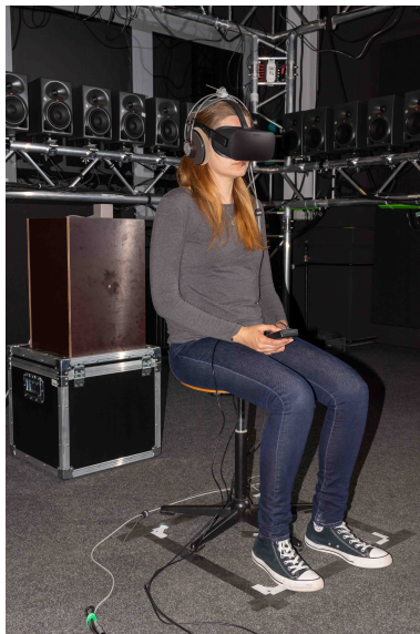
Figure 3.7: Listener in the experimental setup for the localisation experiment.
