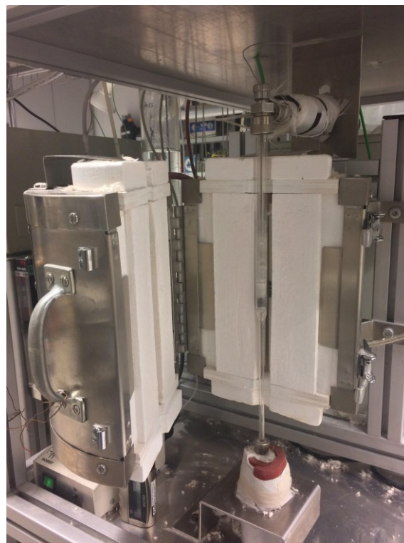
Figure S. 5. The oven with fixed bed reactor for DRM
