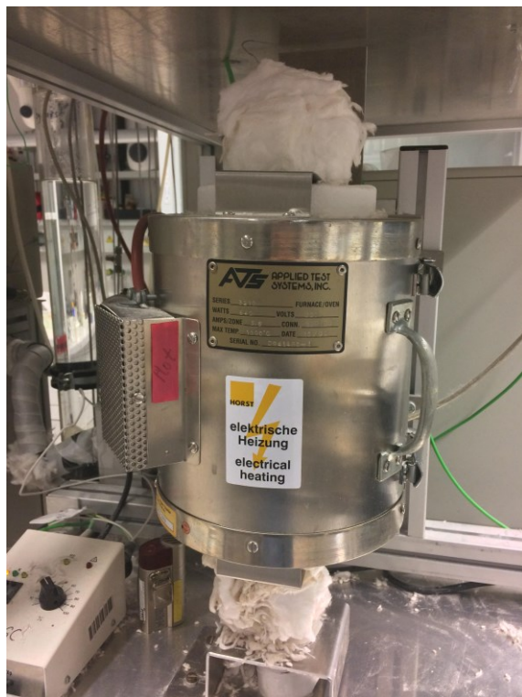
Figure S. 5. The oven with fixed bed reactor for DRM
