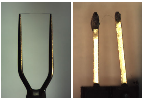
Figure 4.2: Left: LITOS hotwire sensor. Right: HYFLITS hotwire sensor.
