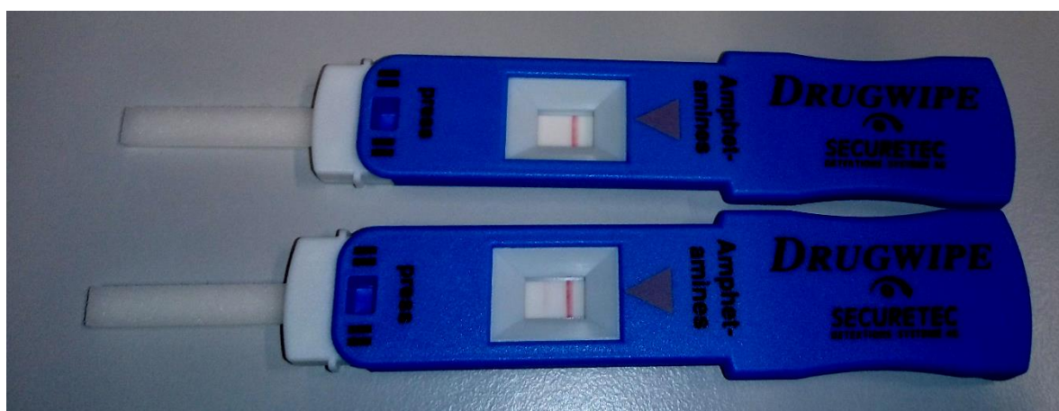
Figure 21: Immunoassay drug tests for amphetamine. Upper test, blind test with no amphetamine and thus only one red mark. Lower test, near LOD with approximately two nanograms of amphetamine. One strong and one weak red mark are visible. A second weak red mark proves the presence of amphetamine.
