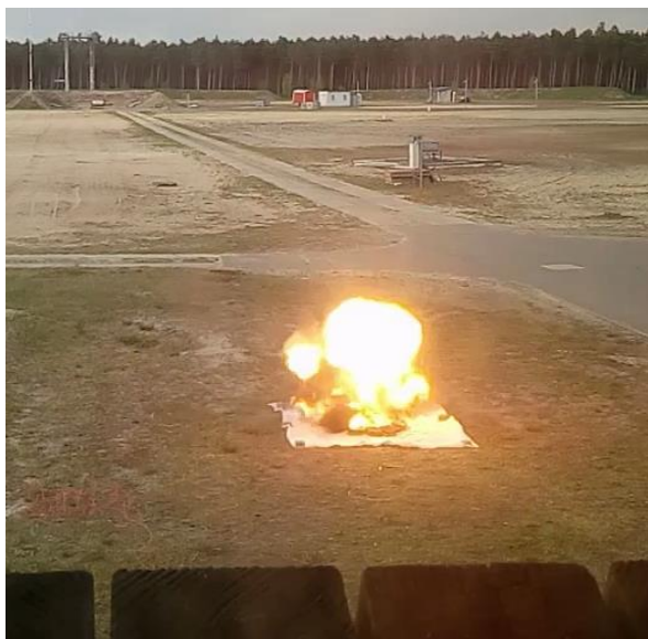
Figure 10: Exemplary detonation of 60 g of SEMTEX, utilised to generate post-blast sample surfaces of this explosive.
