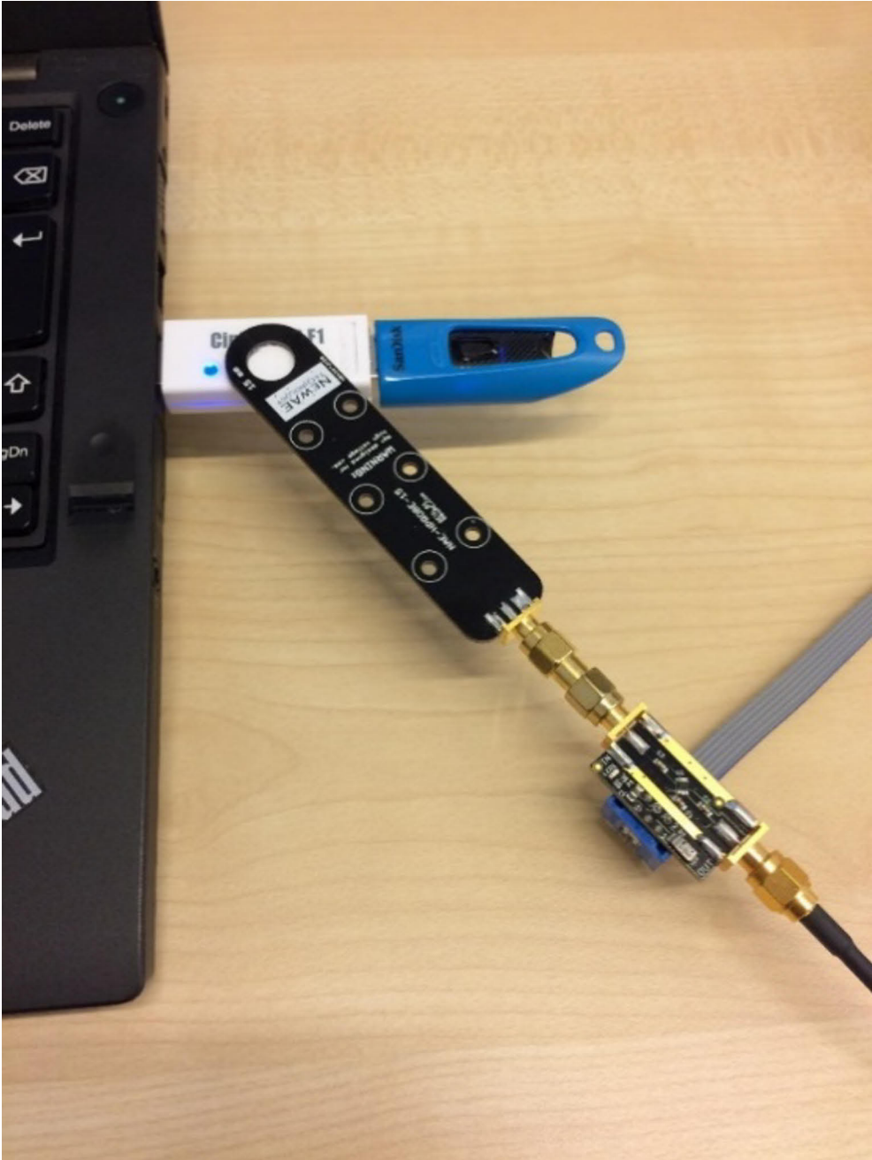
Figure 1. Performing electromagnetic side-channel attack on a commercial AES-256 device
