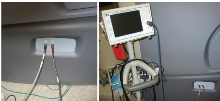
Figure 8. On left is a photo of two different trigger input connectors of the scanner. On right is a photo of ECG monitor that is connected to the ECG trigger input where it can send the trigger information from the R-peak of the ECG-cycle.
