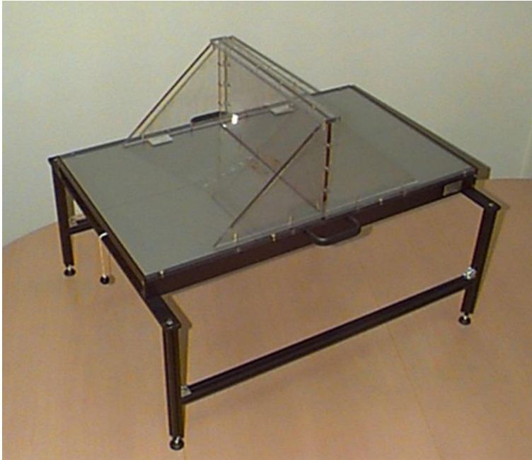
Figure 3. A uniplanar RSA calibration cage with RSA markers inserted in precisely defined positions within the sheets of transparent plastic. Fiducial markers are placed on the flat surface above the X-ray cassettes. Control markers are placed on top of the vertical platform. The same control markers are projected onto each radiograph.
