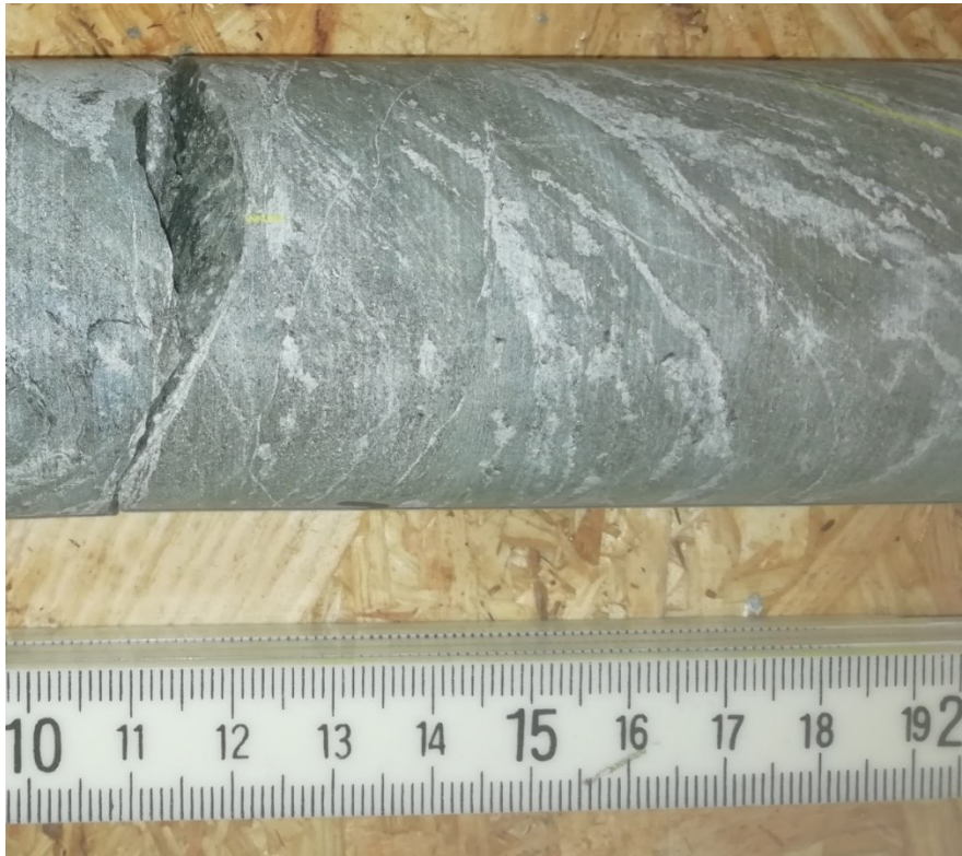
Intensively altered and sheared picrite and characteristic greenish and brownish coloured pervasive alteration. Carbonate veins are oriented mainly parallel to overall foliation.
