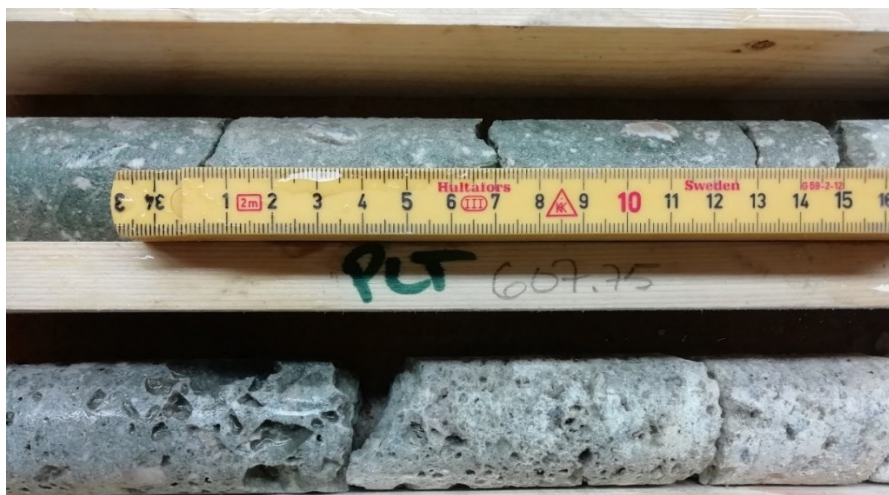
Example of fault breccia found within the footwall basal thrust. Note the angular clasts accompanied with poor sorting and chaotic texture.
