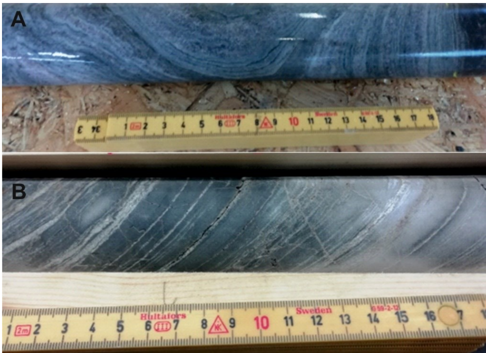
Two subunits of schists; A: Folded Ca-rich schist and B: Intensely sheared Ca-poor schist.
