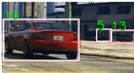
Figure 2.8: Each tracked object gets a unique identity number (shown above the object).
