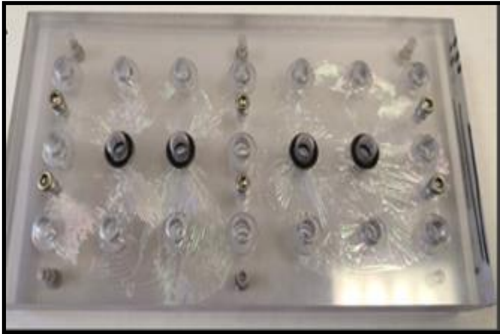
Figure 4.8: The custom cell culture plate with the 2.5 \mu\text{m} Mylar film covers the wells.
