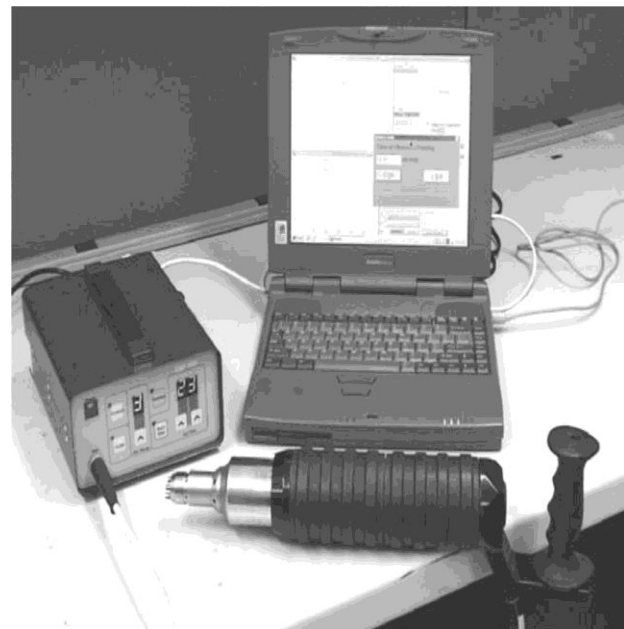
Figure 2. A photo of the computerized complex for receiving an ultrasonic peening from [42].
