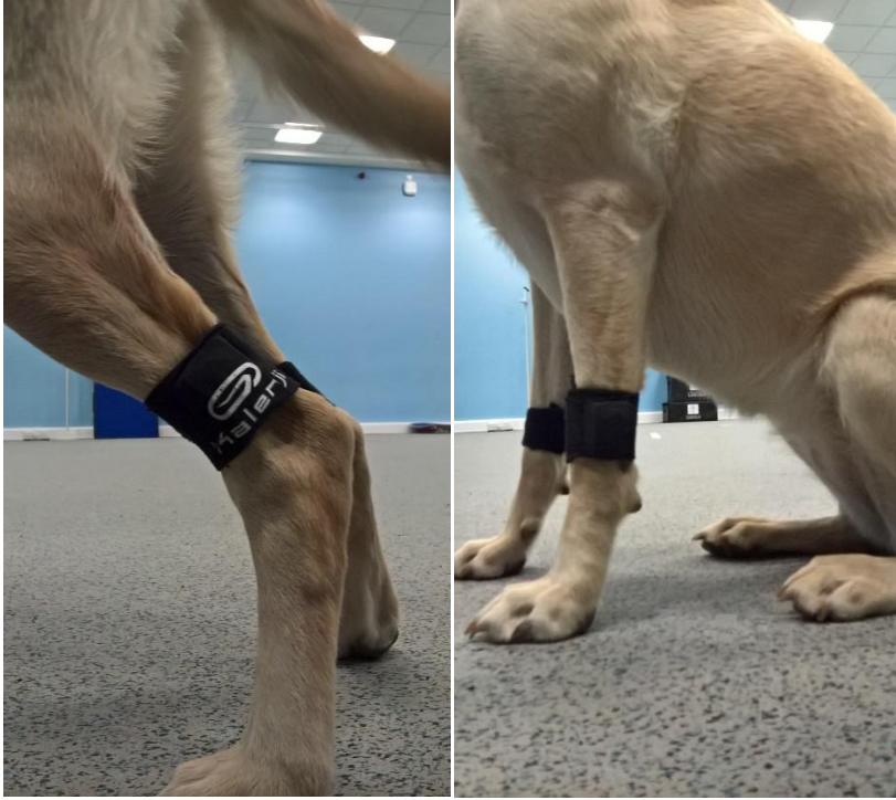
Figure 7:4. Hind and forelimb placement of accelerometers prior to adhesion with bandage wrap
