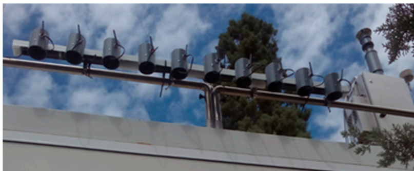
Figure 2. Field calibration of 10 EcoBici devices on the front of an Andalusian Council sampling station in Seville City.
