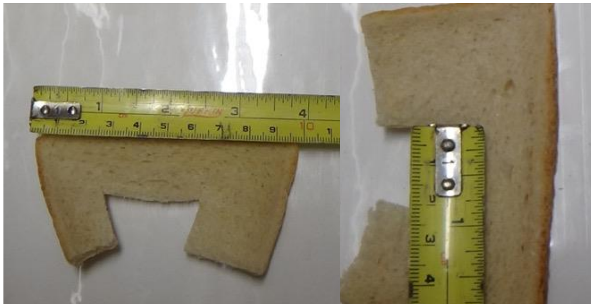
Figure 3.6. A model piece of dried bread to be used in the study; the section cut out of the middle was done prior to drying, thus the square dried distorted.
