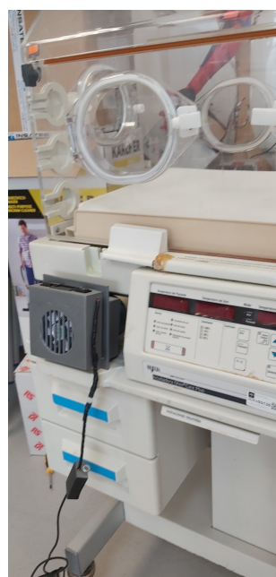
Figure 3. Neonatal incubator with thermoelectric conditioning device.
