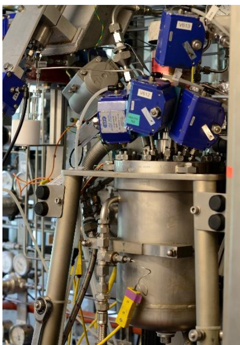
5 L reactor setup for simulating a multistage polymerization process
