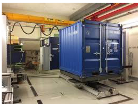
Figure 17. Movable support structure for concept evaluation. Its movement degrees of freedom allow 3D \gamma -ray beam scanning for ‘real-world’ scenarios. Adapted from [153]. CC BY-SA 4.0.
