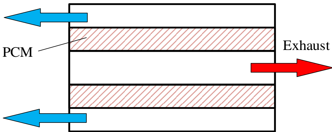
Fig. 4. Diagram of the longitudinal section of the evaporator with LTES
