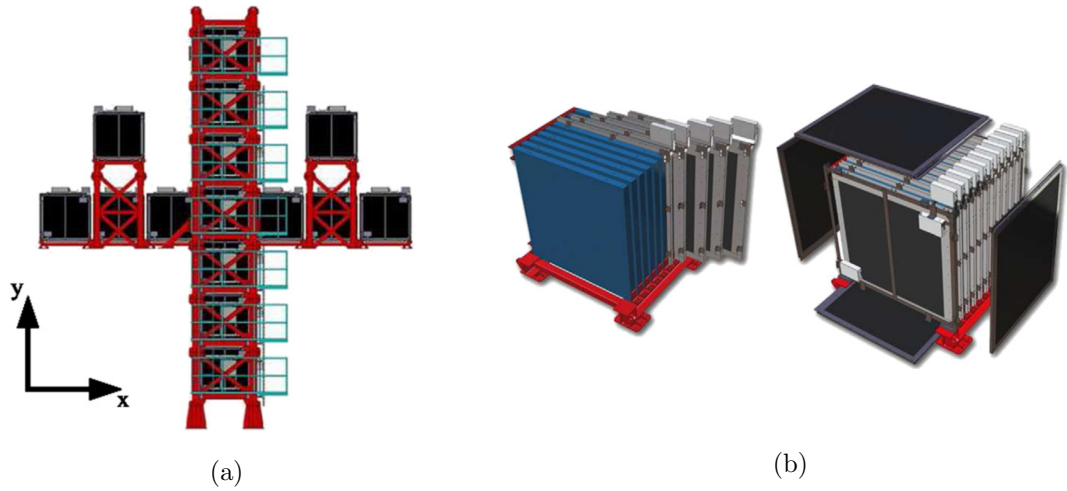
Figure 3.5: Schematic representations of both the INGRID detector (a) and the modules used inside (b). In (b) the left module (blue) shows the tracking planes, the right module (black) shows the veto planes. Taken from [69].
