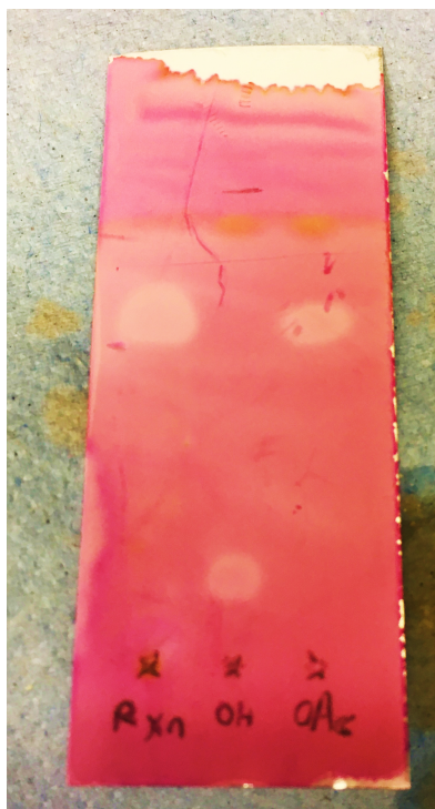
Figure 8. TLC of step A crude reaction mixture after 20 h. Spots from left to right: Rxn = reaction mixture; OH = 1-adamantanol 1 (starting material), OAc = 1-adamantyl acetate 2 (authentic material from a previous batch) (photo supplied by submitters)
