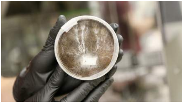
Fig. 17. Mycelia growing on Martian regolith simulant.
