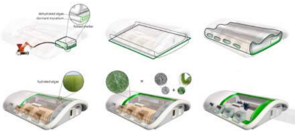
Fig. 11. Fully encased structures self-assemble when water, CO 2 , and heat are added by a robot (image credit: rehouse studio)
