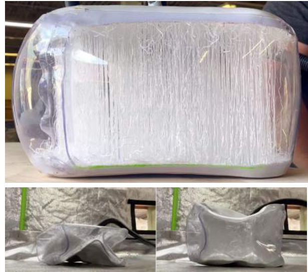
Fig. 16. Drop-stitch inflatable, (image credit: redhouse studio)
