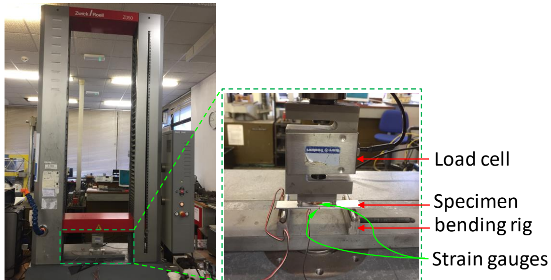
Figure 5: Experimental 4-point bending test setup.
