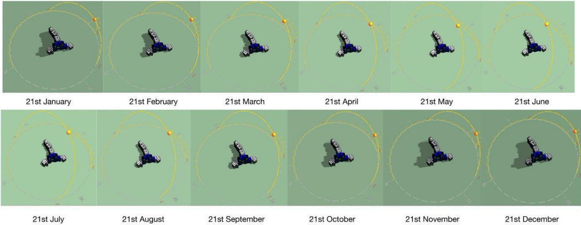
Figure 8. The sun path diagram demonstrates that the southwest-facing block experienced high levels of solar radiation most of the day in July and August 2020.
