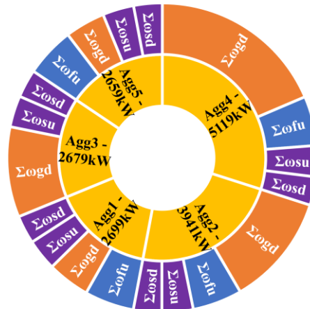
Figure 9. Distribution of the products traded in the market for each aggregator in the imbalance solving scenario. Blue, orange, and purple segments represent FLs, FGs, and BESSs, respectively.
