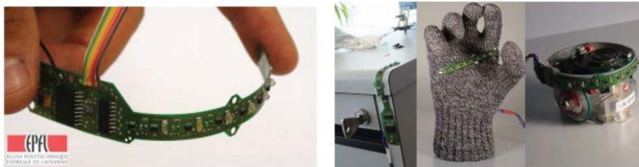
Figure 2.54: Left, image of the Vision Tape in curved configuration; right, examples of integration of the VT onto different substrates (Dobrzynski et al. (2012)).
