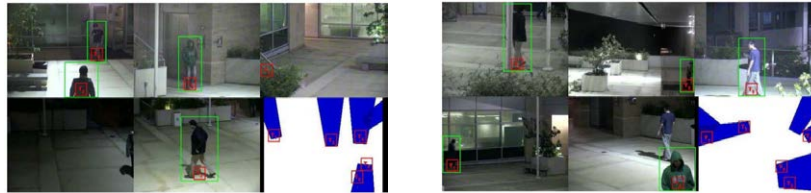
Figure 2.43: Dynamic camera control images. Blue regions mark the FOV; darker regions identify camera overlap in the system developed in Ding et al. (2012)
