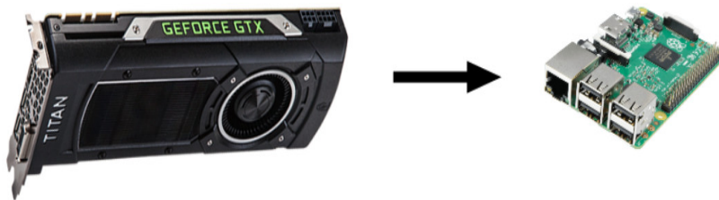
Figure 1.2: Potential hardware architectures to be used in the deployment of artificial neural networks-based computer vision algorithms. Left, high performance Titan X NVIDIA card with a GPU. Right, Raspberry Pi 2 Model B microcomputer.
