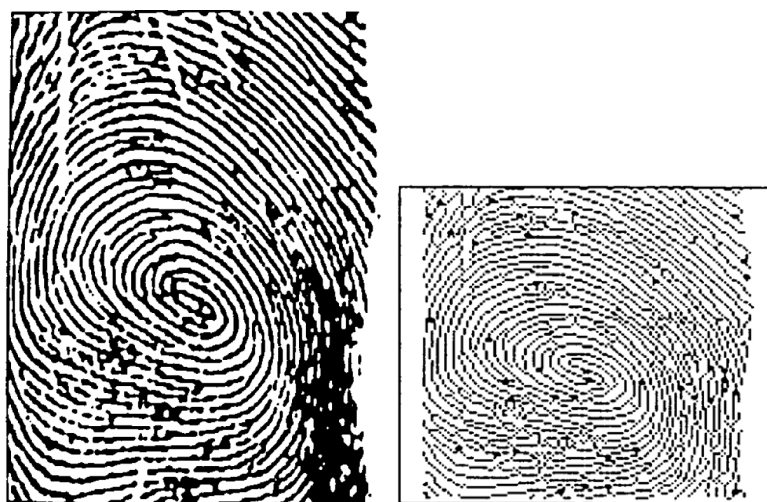
Figure 2.12: Right: Original gray-level fingerprint; left: Feature points extracted from thinned prints (Leung et al. (1991)).
