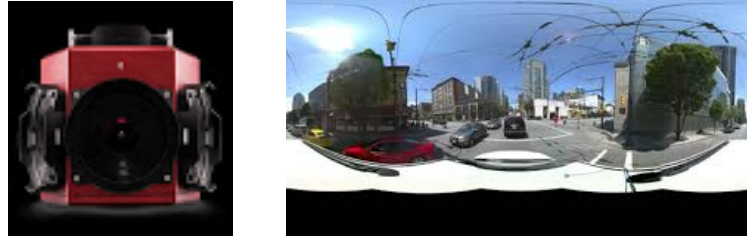
Figure 2.49: Left, image of a Ladybug5+ 360° panoramic camera; right, 360° frame captured by the Ladybug5+.
