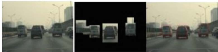
Figure 2.5: Results of two-step detection performed by the combined Haar and HOG feature-based detector in urban traffic (Wei et al. (2019)).
