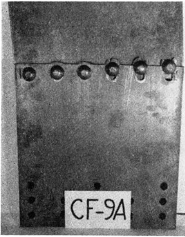
FIG. 5. FAILURE BY TEARING OUT OF RIVETS TO THE EDGE OF OUTSIDE SHEET, SPECIMEN CF-9A
