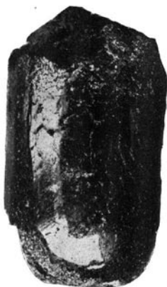
FIG. 12. PHENOL SOLUBLE EXTRACT FROM WIL- LIAMSON COUNTY COAL—AFTER DESTRUCTIVE DISTILLATION.
