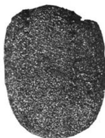
FIG. 11. INSOLUBLE RESIDUE FROM WILLIAMSON COUNTY COAL—AFTER DESTRUC- TIVE DISTILLATION.
