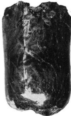
FIG. 9. PHENOL SOLUBLE EXTRACT FROM VERMILION COUNTY COAL—AFTER DE- STRUCTIVE DISTILLATION.
