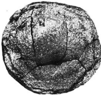
FIG. 17. COKE FROM WILLIAMSON COUNTY COAL WITHOUT PREVIOUS HEATING.
