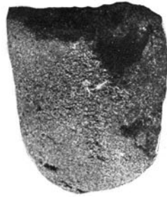
FIG. 8. INSOLUBLE RESIDUE FROM VERMILION COUNTY COAL—AFTER DESTRUCTIVE DISTILLATION.
