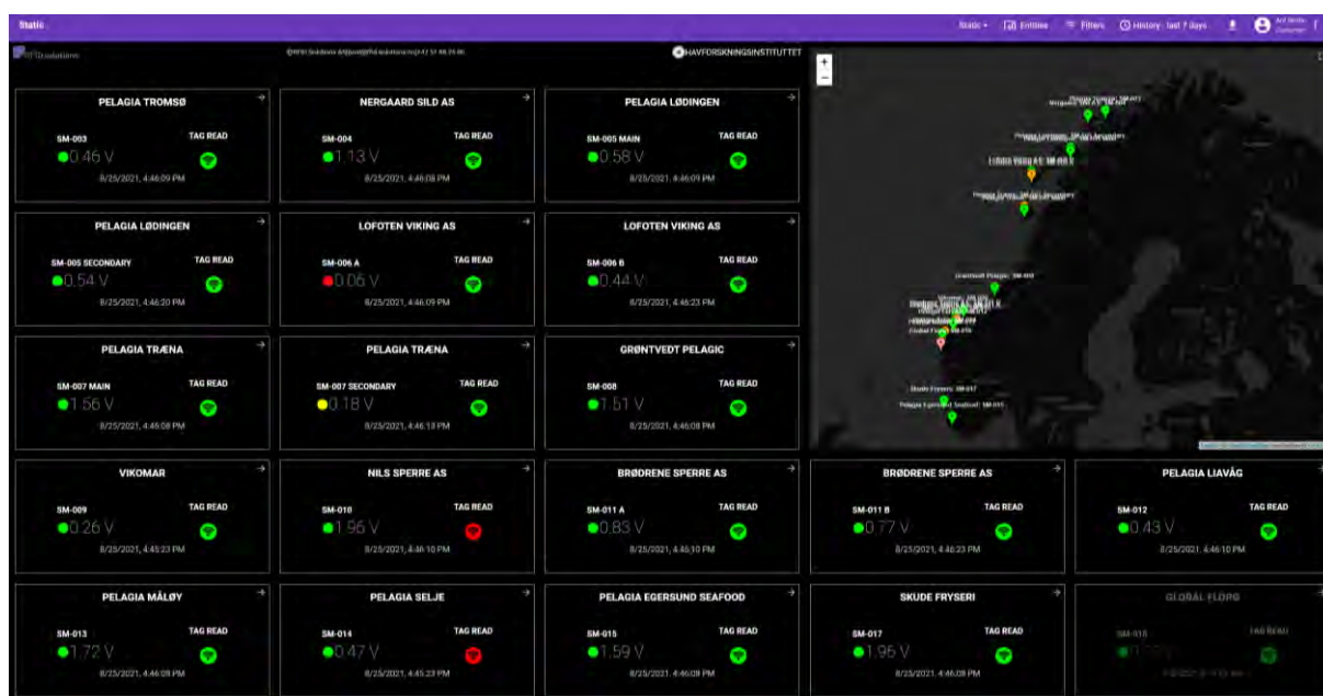
Figure 1. Example of how the new monitoring systems looks like. It follows the traffic light systems, where red implies that we currently may have issues with either voltage variations or reduced efficiency of RFID tags.
