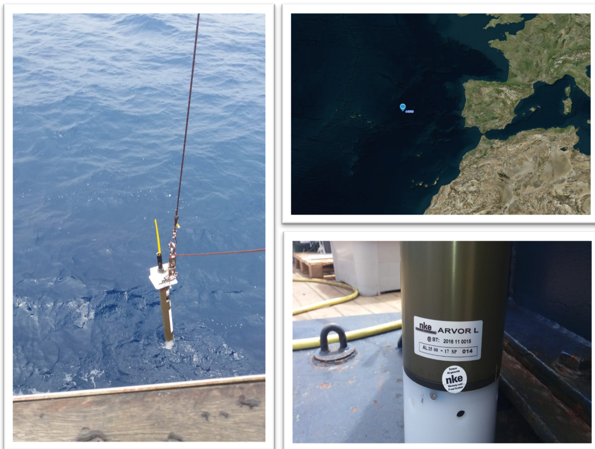
Figure 12 (a), Figure 12 (b) and Figure 12 (c). Deployment maneuver of float WMO 6901265 (a). Deployment location from CLS satellite viewer (b). Serial number and Bluetooth number of the float (c).
