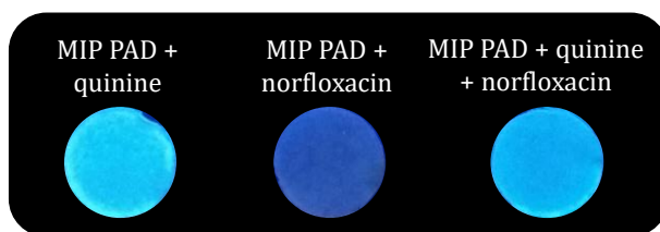
Figure S2. Photographs under ultraviolet lamp of a MIP PAD after extraction of the target analyte (quinine) from an aqueous solution at a concentration of 5 \text{ mg}\cdot\text{L}^{-1} ; MIP PAD after extraction of norfloxacin from a 5 \text{ mg}\cdot\text{L}^{-1} aqueous solution and MIP PAD after extraction of a solution containing both quinine and norfloxacin at the same concentration of 5 \text{ mg}\cdot\text{L}^{-1} .
