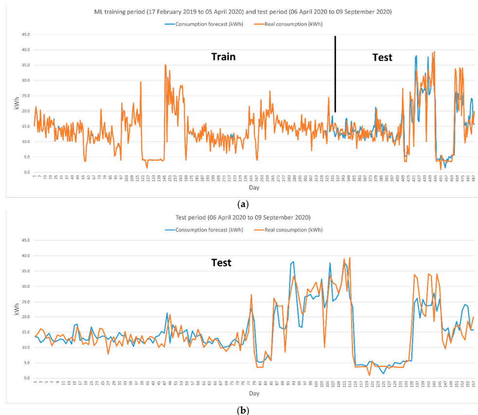
Figure 25. Comparison between estimated consumption and actual consumption in Wh. (a) ML Table (17 February 2019 to 5 April 2020) and test period (6 April 2020 to 9 September 2020). (b) Test period (6 April 2020 to 9 September 2020).
