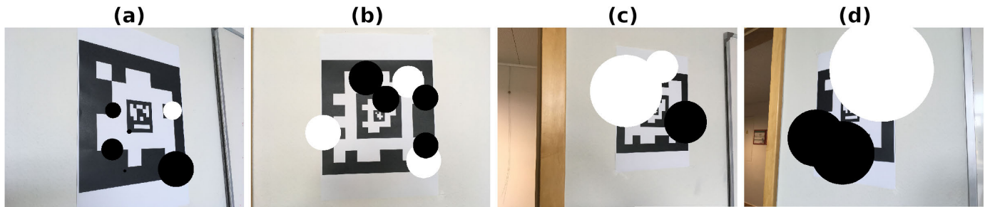
FIGURE 13. Some of the images employed to test detection under occlusion. Different levels of occlusion are synthetically added to the images: (a) 11.29%, (b) 33.19%, (c) 53.92%, (d) 73.37%.
