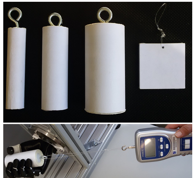
Fig. 5. Plate (60x60x5 mm, 49 g) and cylinders S, M, and L (100 mm length, from left to right: diam. 22/32/50 mm, 28/48/48 g) used for the slip resistance test.
