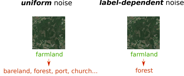
Fig. 2. Two types of label noise are considered in this paper. (Left) Uniform noise: a true label is flipped into other labels with equal probability. (Right) Label-dependent noise: a true label is more likely to be mistakenly labeled with a particular class.
