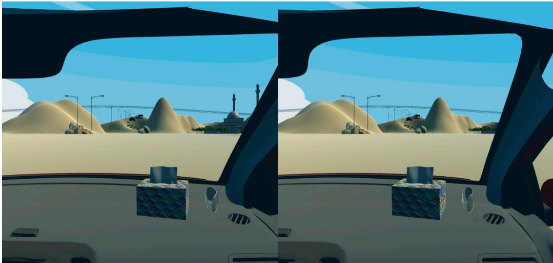
Figure 2. Snapshot of the simulation as seen from the front passenger's position. The two images correspond to the right and left eye, since the VR application is a stereoscopic software.
