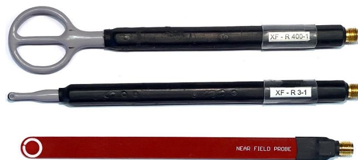
Figure 14. Photograph of designed NFP PCB and XF-R 3-1, XF-R 400-1 probes.
