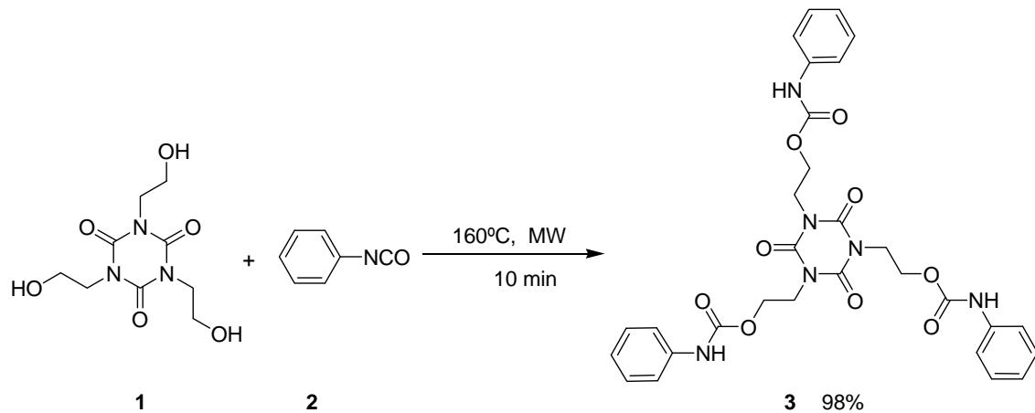
The same reaction conditions were optimal for the coupling of α-naphthylisocyanate with THECA, yielding the corresponding tris-naphthylcambamate in 97% yield. Similarly to **3**, this compound showed peaks in the <sup>1</sup>H-NMR spectrum at δ 4.11 y 4.31 ppm for -CH<sub>2</sub>CH<sub>2</sub>- chains and δ 9.16 ppm for N-H.
