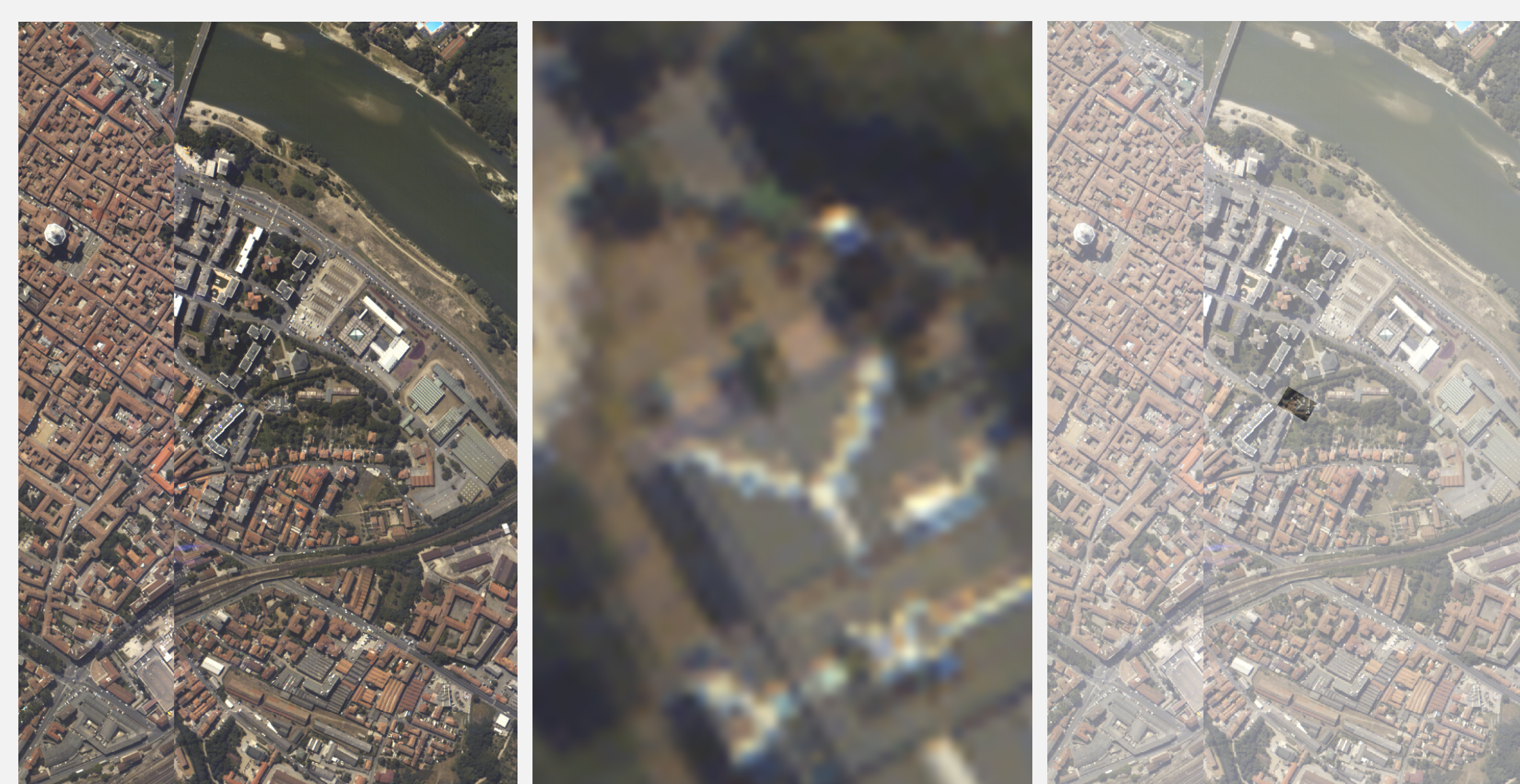
Figure: Example of registration considered in this work: a) Reference image (size 1096 \times 715 ), b) Target image, and c) Result of the registration process showing the correctly registered superposition of the reference and target registered image (scale 23.0\times and rotation angle 60^\circ ).
