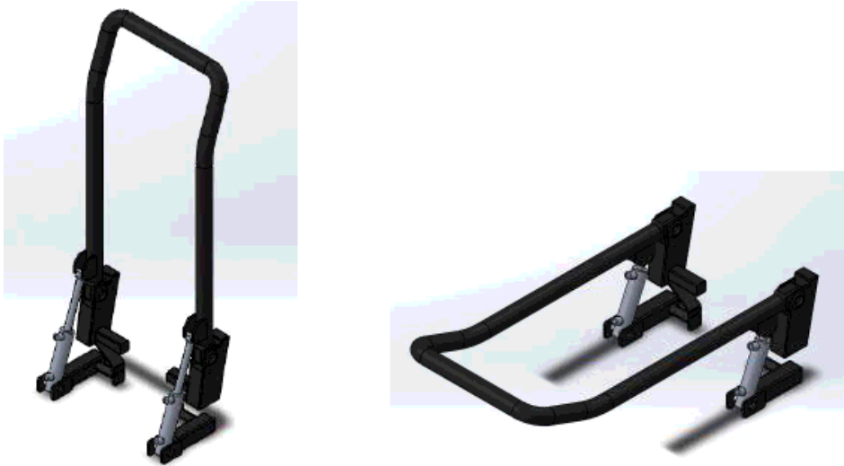
Figure 3. 3D model of ROPS components. (left) up position, (right) down position.
