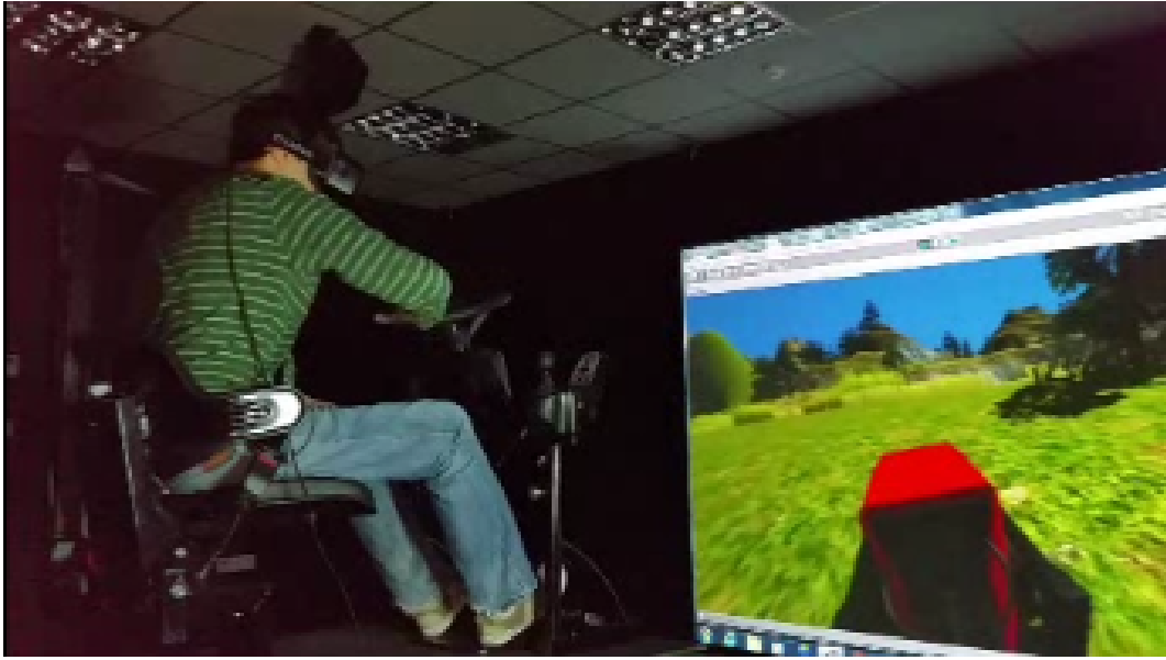
Figure 6. Participant driving the simulation motion platform.
