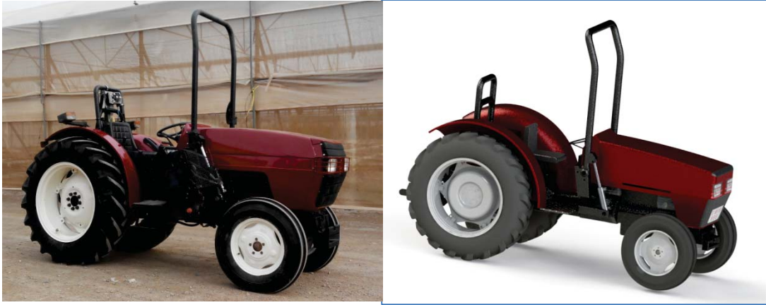
Figure 1. (left) real CASE IH-2120 tractor. (right) 3D model of CASE IH-2120 tractor.
