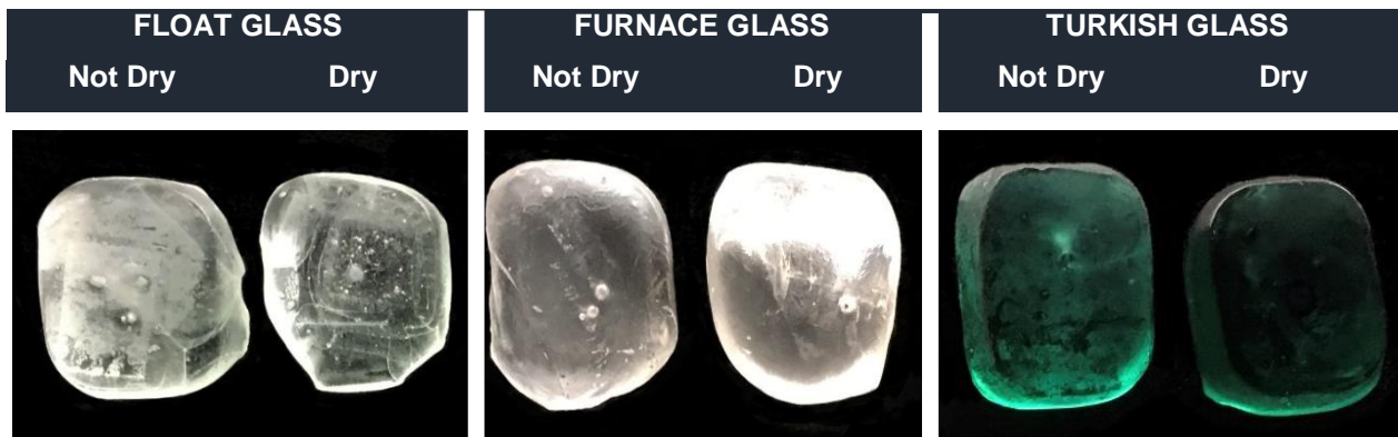
Figure 36 Samples of glass with drying moulds on the right and without drying moulds on the left.
