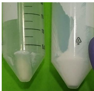
Figure 3.1 – ZnO NPs obtained using NaOH with different solvents: methanol (on the left) and water (on the right)
