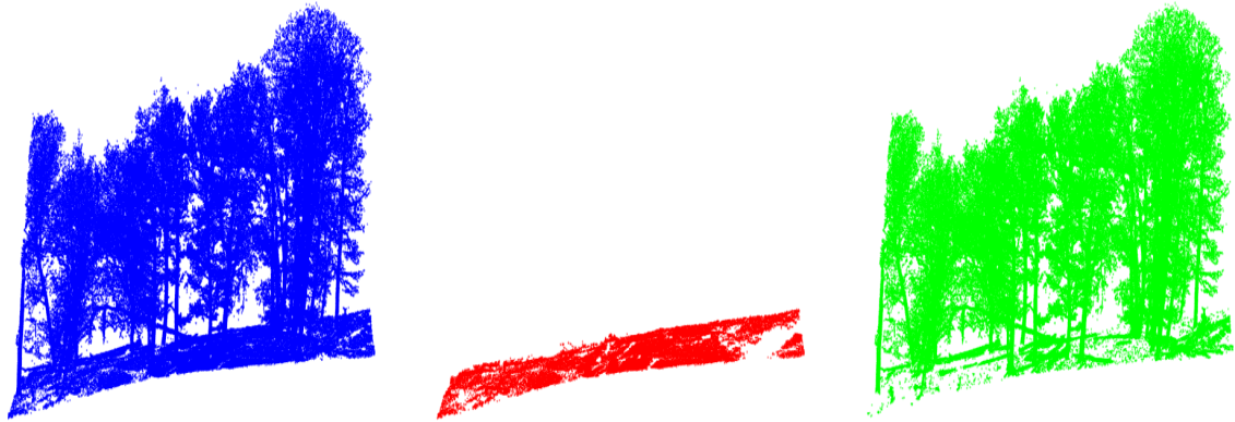
Figure 4.4: Original high resolution point cloud of figure 4.2. From left to right: Original point cloud, ground returns classified by the progressive morphological filter and again, vegetation cloud, resulting from the subtraction of the ground returns from the original sub set.
