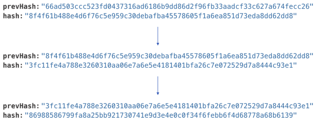
Figure 3.6: Blocks always have an unique hash as well as the previous block's hash
